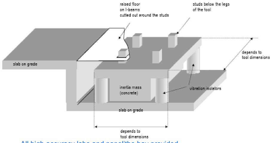
All high accuracy labs and nanolitho bay provided with pitsfor inertia mass placement
